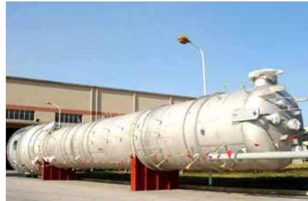
萃取塔 Extraction tower
